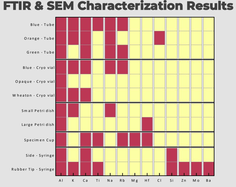
The chart shows every element found within each lab plastic used. Al was prevalent within every sample. The syringe showed both the side material and tip to contain the most contaminants.
