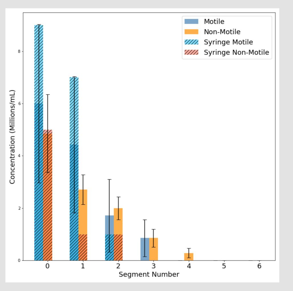
Motile and non-motile sperm cells were recorded and averaged. The graph shows a sample test exposing sperm cells to the syringe for 30 minutes. The initial concentration was higher at the waste port, and decreased dramatically as the segments went on compared to the average unexposed tests.
