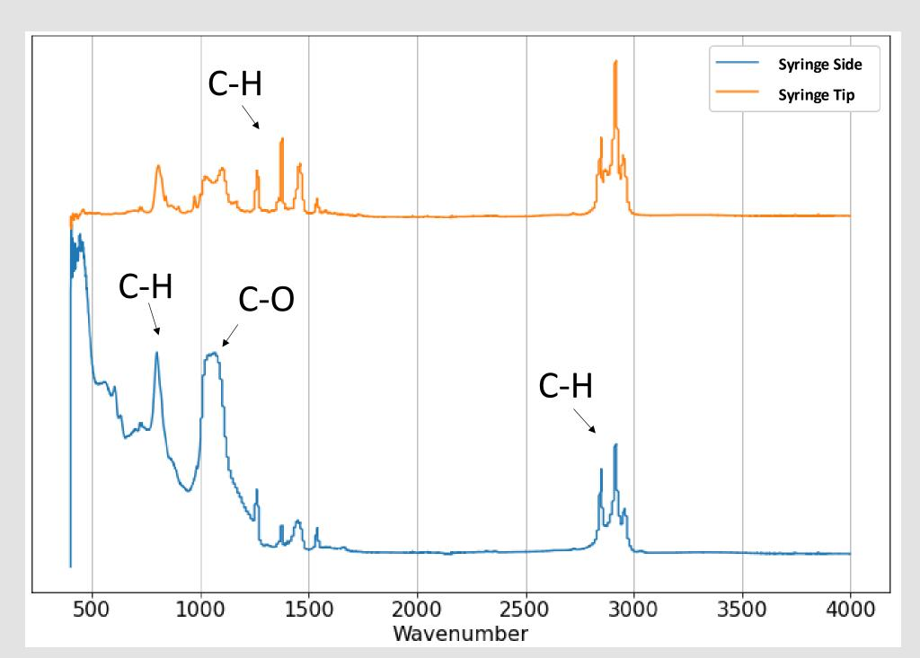
The graph above shows the results of the syringe side and tip. The side of the syringe contains peaks similar to most of the lab materials used. However, the tip is a unique material unlike any other samples.
