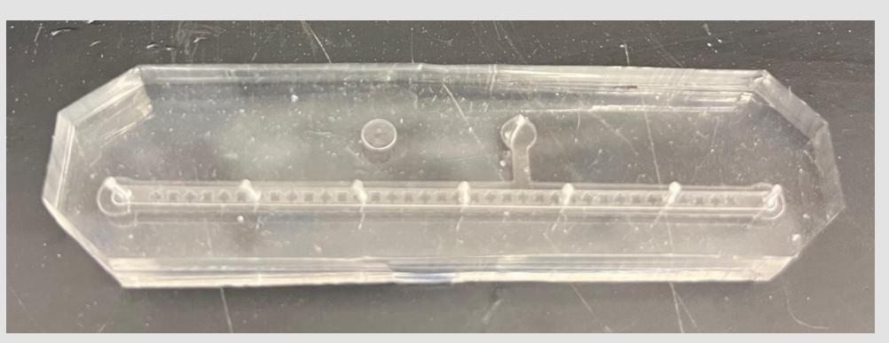
The microfluidic racetrack above has 6 segments excluding waste and HTF entrance that were utilized in the experiment.
